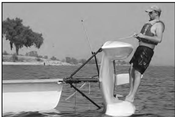
8. As the boat comes up, slide into the water and grab the hull coming over your head. **Don't let the hull hit your head.** Control the speed of the hull coming down. If it were to come up quickly, the momentum of the mast would throw it over to the other side.
