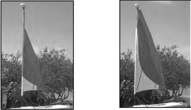
Shown here are examples of two different reefed positions. Keep in mind that the higher the wind, the more the sail should be reefed. Also, for best performance, adjust the reefing position so that the mast float faces forward.
