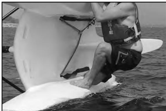
9. **Once the boat is upright, be sure to hang on to the boat. After the sail is back up, the boat could sail away from you.** If the wind is strong, it may be necessary to hold the boat down to prevent it from re-capsizing.
