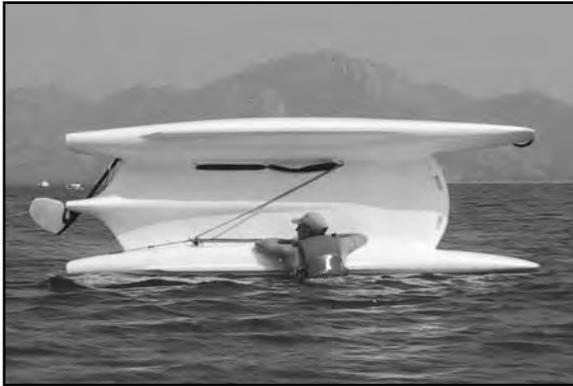
2. Orient the boat so that the wind is coming to a 45 degree angle to the mast (see diagram to the right). Doing this will allow the wind to help lift the boat out of the water.
