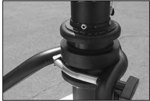
2. Align the boom clip to the groove and give a strong push forward. The clip will flex slightly and snap around the bearing.
