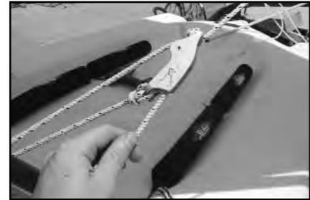
7. Attach the mainsheet hook to the padeye at the bottom rear of the boom.
