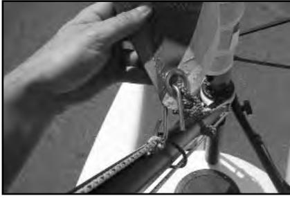
5. The line that runs the length of the boom is called the outhaul. It controls the location of the clew of the sail. By pulling on the outhaul line, it will move the clew of the sail out on the boom away from the mast.
