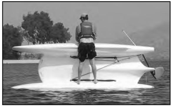
It is actually possible to right the boat without the righting line system. Grab hold of the hull or hiking straps and lean away from the boat to pull the sail out of the water.
