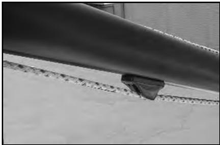
To furl the sail, uncleat the outhaul line and pull in on the mast furling line. Note that as you pull in, the boom is going to rise upward.
